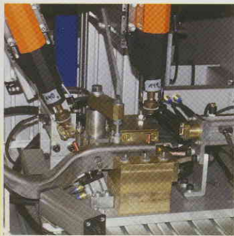
Dual head facility enables simultaneous welding of studs
