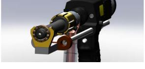
the foot piece to be adjusted to remove any binding between the stud and ferrule. Once these conditions are satisfied, you are now
